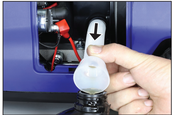
Figure 25 – Draining the Engine Oil
