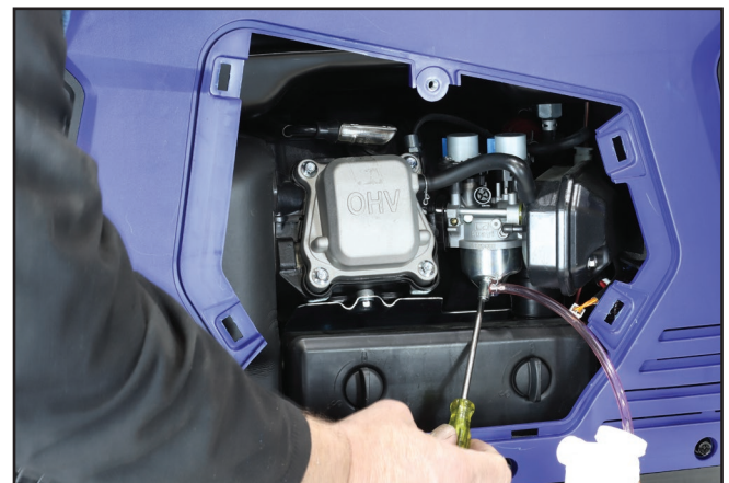
Figure 38 – Draining the Carburettor
