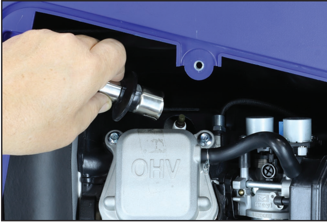
Figure 31 – Removing the Spark Plug Boot
