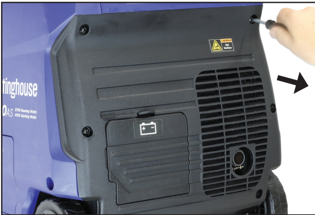
Figure 34 – Removing the Muffler Access Cover
