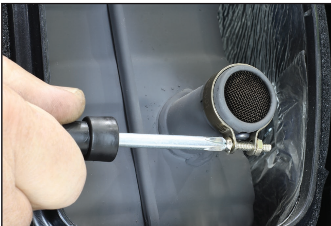
Figure 35 – Removing the Spark Arrester Band Clamp
