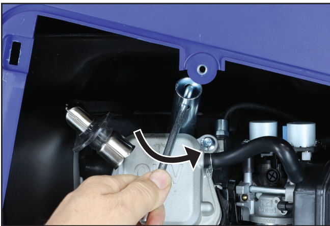
Figure 32 – Removing the Spark Plug
