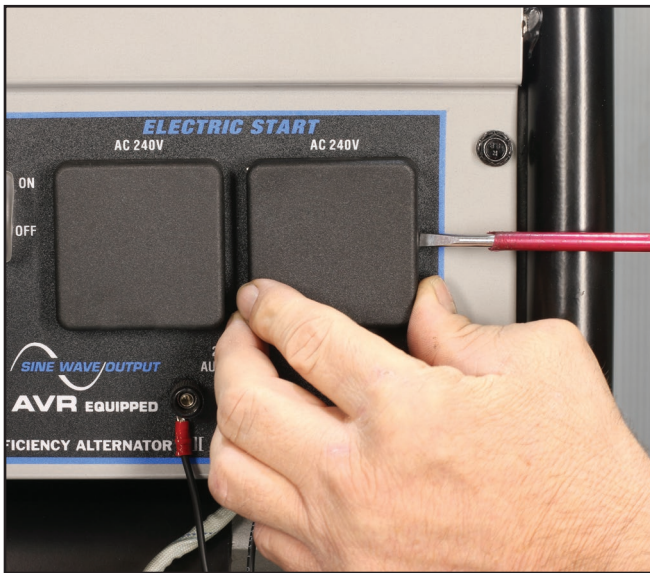
Figure S3 – Removing the 240-Volt AC Socket Cover
