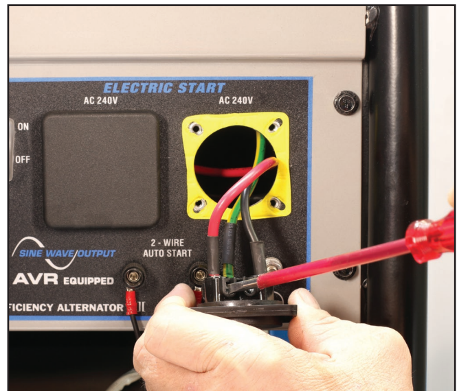
Figure S6 – Disconnecting the 240-Volt AC Socket
