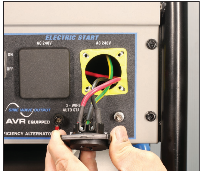
Figure S5 – Withdrawing the 240-Volt AC Socket
