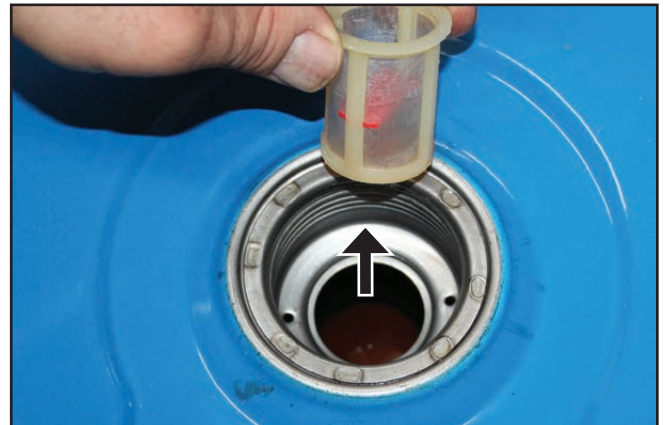
Figure 38 – Removing Fuel Strainer.
