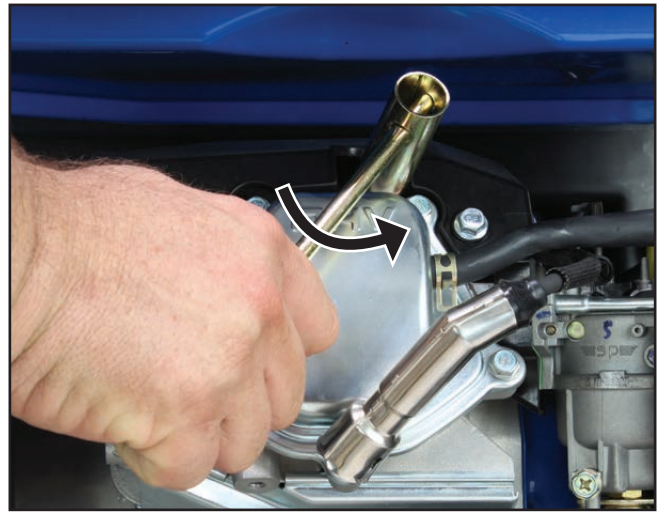
Figure 44 – Removing Spark Plug
