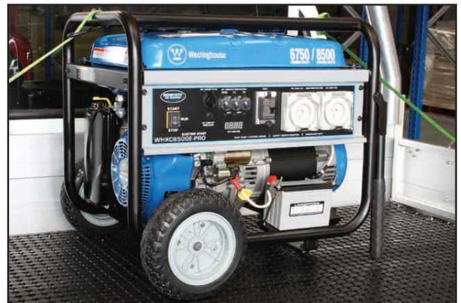
Figure 25 – Generator Restraint for Transport
