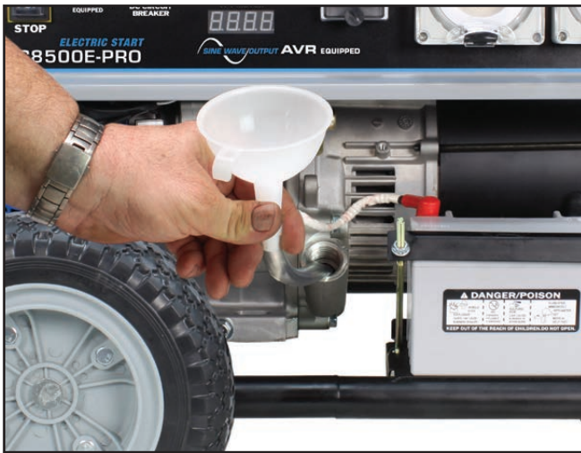
Figure 28 – Adding Engine Oil
