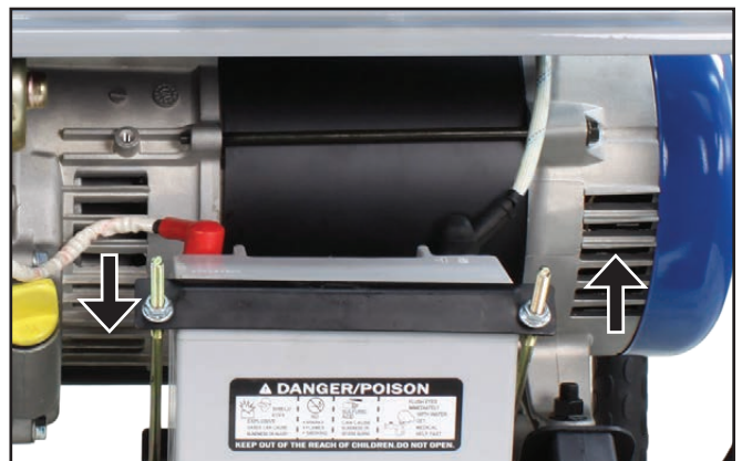
Figure 49 – Alternator Cooling Air Inlet and Outlet Ports
