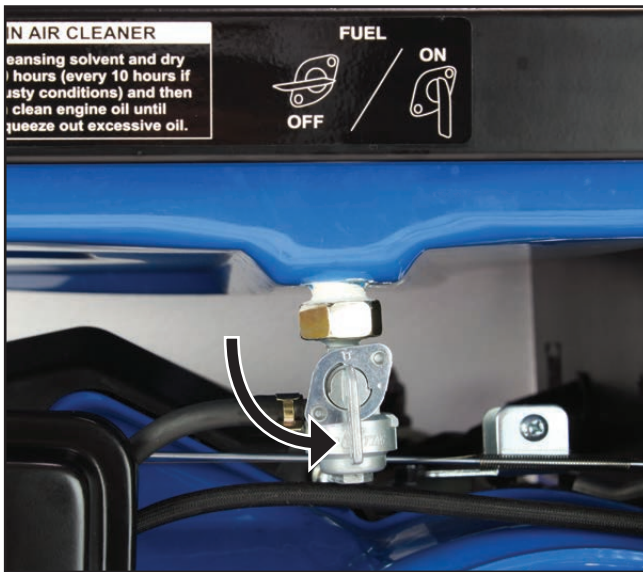
Figure 15 – Fuel Shutoff Valve in the ON Position
